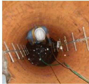
Vertical Scanning of a Condensate Tube
