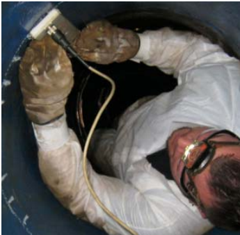
Through Wall Spool Scanning through an Enecon Coating Product
