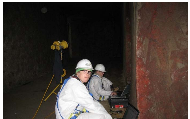
Dual Internal BEM Scanning of large diameter piping at Oyster Creek, Nuclear Power Plant.
